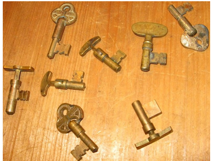
A selection of specialized pocket-door keys. Many have tops that fold over, so they can be left in the lock and not protrude when the doors slide into the wall.
